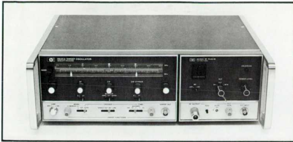
Fig. 1. Model 86290A is a new RF plug-in for Model 8620A Sweep Oscillator. Four frequency bands are selectable by front-panel controls: 2-6.2, 6-12.4, 12-18, and 2-18 GHz. The combination is the most compact broadband sweeper currently available.
